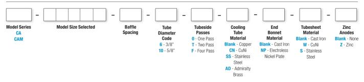
CA = ANSI/ASME shell side flanges; NPT tubeside bottom connections (two & four pass); ANSI/ASME flanges on tube side (one pass).
