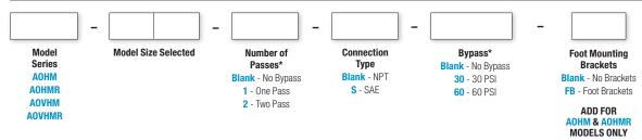
AOHMR - Internal pressure bypass included
